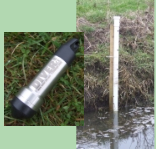
Diver and typical mounting (suspended by stainless steel cable from a screw lid on 40mm diameter plastic drainage pipe)
