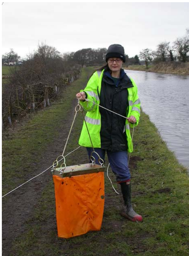
Fig. 27 The 'heavy dredge' used to collect unionid mussels on the Shropshire Union & Llangollen Canals
